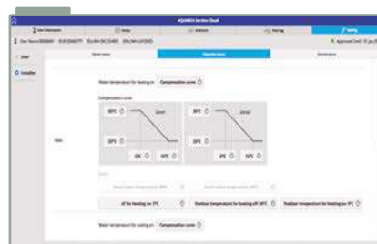
Settings tab. Most of the user and installer settings can be done remotely.
