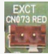
Cable with force thermo OFF/leakage detection.
